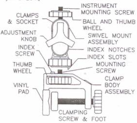
The Universal Mounting Clamp is used to attach the AX300 Oxygen Analyzer or MX300 Oxygen Monitor to IV poles, ventilators and other objects up to 1 ½ inch thick. The Mounting Clamp offers 360—degree rotation and 180—degree movement in all directions providing maximum flexibility in selecting a mounting site.
