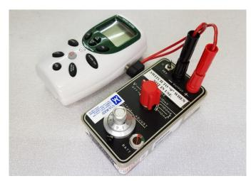
2) Set the Microcal to 100 mV scale and the polarity switch to NORM.
