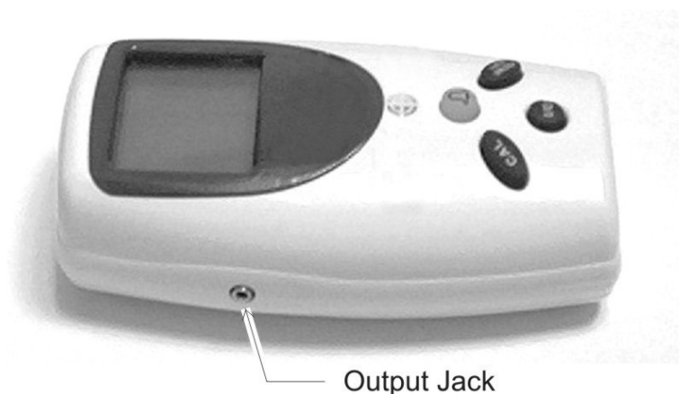
Figure 2-8: 0-1 VDC or RS 232 Digital Output Port
