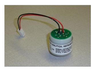
2) Using a soldering iron, remove the black and red wires.
