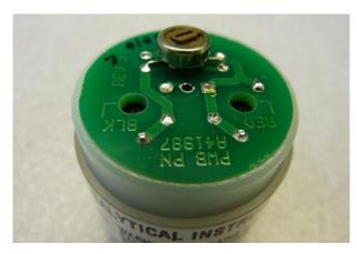
3) Using the flat edge of a Stanley knife, remove a small area of surface lacquer from in front of the solder contacts.
