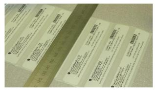
10) Remove the Teledyne label (R-33S1) and replace it with the Vandagraph (D-40) label with the same serial number.
