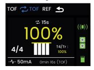
The number of responses detected (TOF count) is displayed as an X/4 ratio (X being the number of muscle response detected).
