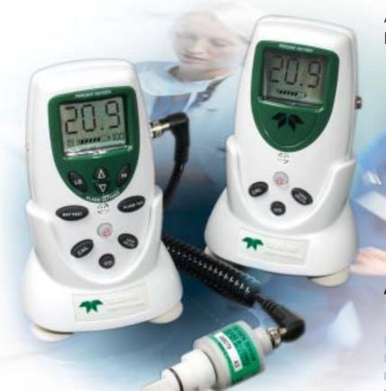
AX300 **oxygen analyser** and MX300 **oxygen monitor**.
