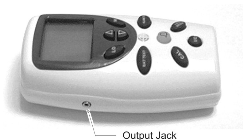
Figure 2-9: 0-1 VDC or RS 232 Digital Output Port
