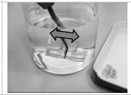
4. Rinse the both items in at least 500ml water (preferably fully demineralized water); Swirl/Move the both items back and forth for at least 1 minute. Remove and place the items on a clean surface and let them drain completely.
