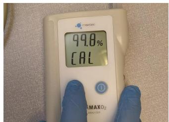
10) Verify the air calibration. Connect the inlet tubing to a source medical air. Allow gas to flow at 2lpm. Record this value on the certificate.
