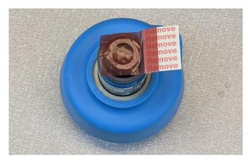
2) Affix the flow divert to the thread on the bottom of the sensor.
