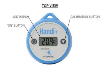
1) A protective film covering the threaded sensor face must be removed and the sensor allowed to "breath" for at least 30 minutes.
