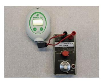
2) Set the Microcal to 100 mV scale and the polarity switch to NORM.
