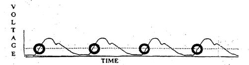
Point of pulse detection at which signal voltage crosses a predetermined threshold
