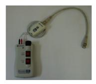
NOTE: The Microstim DB3 Tester reduces the output of the Microstim DB3 by a factor of 100 in order to facilitate easy testing.
