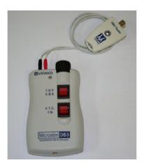
3) Depress each of the Microstim DB3 function buttons in turn. When a function button is pressed and held there should be audio output in conjunction with illumination of the green LED indicator on the Microstim DB3 (refer to page 2. Modes of Stimulation). The output can be verified by observing if the red LED indicator on the Microstim DB3 Tester is also illuminated in synchronization.
