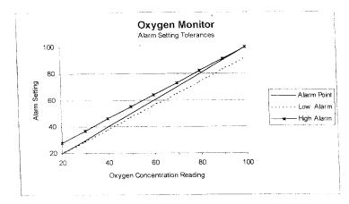
The instrument will alarm at any oxygen concentration below 18%.
