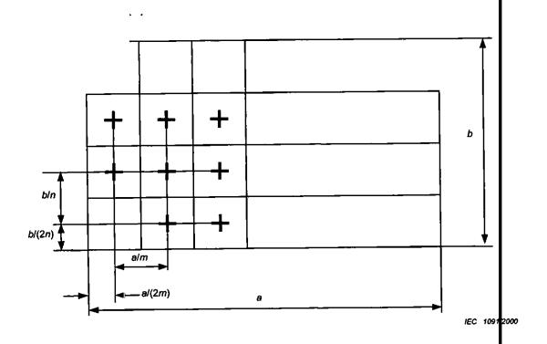
NOTE m, n are the number of partial surfaces in the direction of length a and width b.
