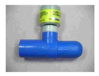
Oxygen sensors are designed to work best in very low constant flowing gas at steady temperatures. The ideal condition is therefore a still gas at 1Bar.
