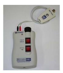
3) Depress each of the function buttons in turn. When a function button is pressed and held there should be audio output in conjunction with illumination of the green LED indicator on the Microstim DB3. The output can be verified by observing if the red LED indicator on the DB3 is also illuminated in synchronization.
