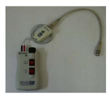
NOTE: The DB3 Tester reduces the output of the Microstim DB3 by a factor of 100 in order to facilitate easy testing.
