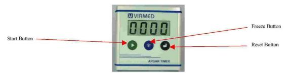
The Viamed Apgar Timer is a battery powered digital timer with preset audible timing indications
