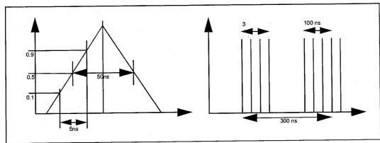
The spike frequency is 5 KHz. The generator produces bursts of spikes during 15ms every 300ms.
