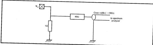
The 1 ohm resistor is inserted into the main GND wire, this means between power supply, decoupling capacitor and pin load on one side and IC GND plus oscillator load.
