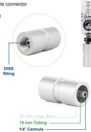
The 3-in-1 Adapter is designed to be compatible with multiple sizes of commonly used medical tubing. It provides the user with the option to connect 22 mm Large Bore, 15 mm or 1/4" Cannula to any DISS fitting such as commonly used flow meters.
