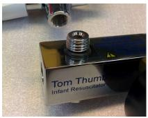
10) Screw the flowmeter onto the inserted flowmeter bolt ensuring the flowmeter is straight in comparison to the body block. Use the 5/8 AF spanner to tighten.
