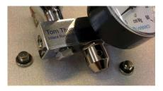
13) Place a thin O ring over the thread of a blanking bolts.
