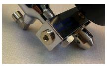
15) Screw into the right hand threaded hole on the bottom face of the body block. Use a 5mm Allen key to tighten.
