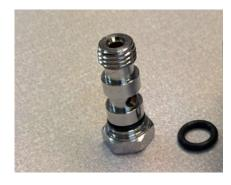
9) Push a thick O ring over the top thread of inserted flowmeter bolt.
