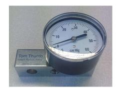
6) Line the thread of the right angle adapter with two complete layers of PTFE tape.
