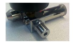
19) Attach the spacer block to the body block using 2x M4x10mm hex drive bolts. Use a 3mm Allen key to tighten.
