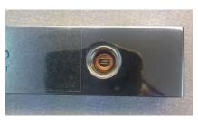
5) Screw the pressure gauge in the single threaded hole on the front face of the body block. The gauge should appear straight in comparison to the block and not able to be removed without the aid of tools. Use 5/8 AF spanner to tighten.
