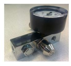
13) Place a thin O ring onto the 10mm inlet.
