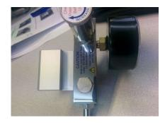
23) Affix the address label to the underside of the pressure gauge.
