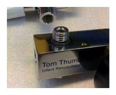
11) Screw the flowmeter onto the inserted flowmeter bolt ensuring the flowmeter is straight in comparison to the body block. Use the 5/8 AF spanner to tighten.
