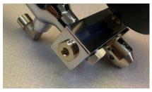
16) Screw into the right hand threaded hole on the bottom face of the body block. Use a 5mm Allen key to tighten.
