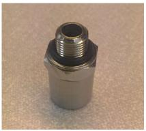
20) Screw the 15mm outlet into the threaded hole in the right face of the body block. Use 5/8 AF spanner to tighten
