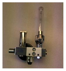
22) Attach rail clamp to the spacer block using 2x M4x10mm hex drive bolts. Use a 3mm Allen key to tighten.
