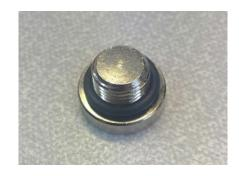
15) Screw the blanking bolt into the left hand end hole of the body block. Use a 5mm Allen key to tighten.
