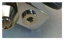
17) Place a thin O ring over the thread of the adjustable valve.
