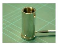
6. Gradually turn the adjustable valve screw until the threaded hole in the internal stop is visible through the slot in the body. Fix in place with a centre screw, fully flush with the body.
