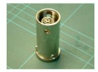
8. Lightly grease the spindle of the valve seat and insert through the spring. Ensure that the spindle engages with the hole in the adjustable valve screw.
