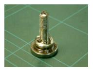
2. Screw on the adjustable valve internal stop, <sup>3</sup>/<sub>4</sub> down the base thread.
