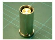
9. Screw on the adjustable valve seating.
