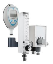
INSERT OXYGEN ANALYZER WITH SENSOR DIVERTER INTO THE SENSOR PORT TO MEASURE THE DELIVERED GAS FROM THE BLENDER.
