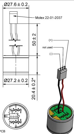
\*Sensor housing height, without PCB
