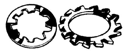
Shakeproof washers are designed with tooth forms designed to indent and grip on the bearing surfaces when tightened down to provide a locking action resistant to loosening by vibration. They are normally made from carbon steel or stainless steel.
