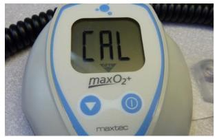
7) The analyser should display 20.9 when tested in air.
