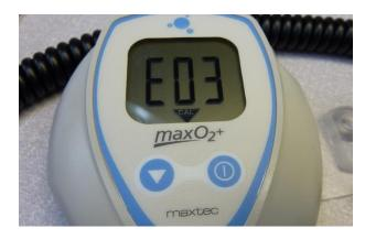
6) Press the calibration button until CAL is displayed.
