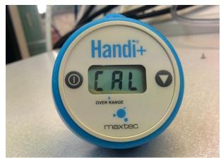
6) The analyser should display 20.9 when tested in air.
