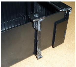
13) Enlarge the pilot hole to fit the power button. Cut in a small notch to act as a key for the power button.
