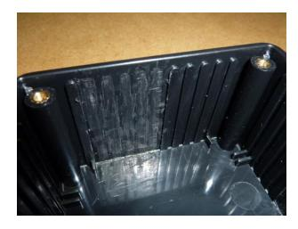
Using a chisel, remove guides 6 and 7 from the side of the case. This is where the power button will be placed.
