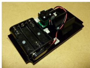
30) Insert the chassis plate into the case ensuring that the orientation is correct.
