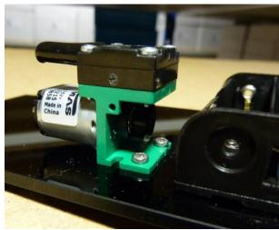
25) Using the pan head machine screws (PN\*\*\*\*\*)., with bolts on the underside (PN\*\*\*\*\*)., affix the sensor holder (PN:CP-1253) to the chassis plate insert.
