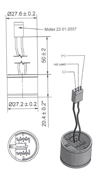
General tolerances ISO 2768-c \*Sensor housing without PCB
