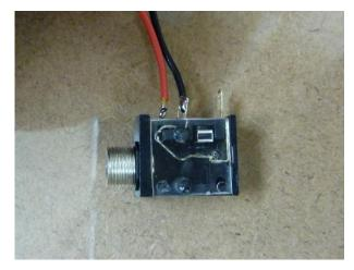
4) Solder the revision 2 sensor input connector to the black and red wires.
