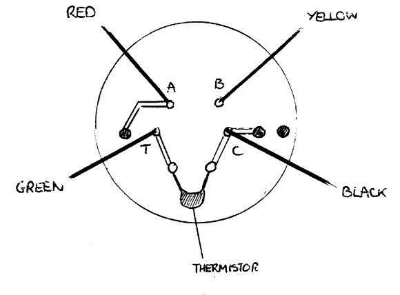
VIEW OF PCB IN SENSORHOLDER FROM THE BACK (THE PINS WHICH CONTACT WITH THE CELL PARE ON THE OTHER SIDE OF PCB)
