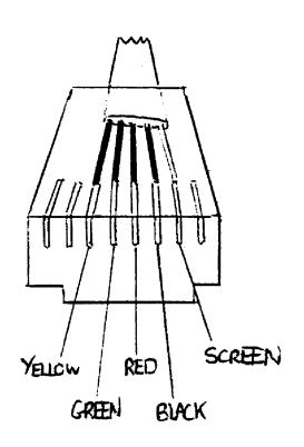
VIEW OF PLUG LOOKING INTO END OF PLUG WITH SPRING-LATCH TO BOTTOM
