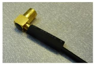
33) Using a heat gun, shrink the heat shrink into place. Ensure that the heat shrink is flush to the connector body.
