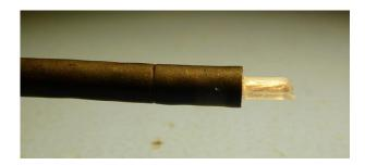
6) Remove the clear plastic cable inner, as shown. Ensure that there are no excess strands of the outer shield near the wire core.
