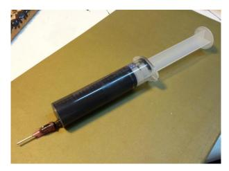
27) Fill the connectors with the resin. Try to avoid leaving air gaps.
