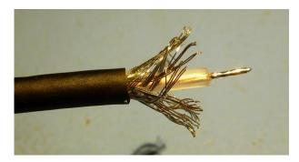
10) Feed the solder through the cable entry and into the slot of centre pin.
