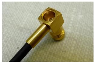
17) Place the crimp into the large hole of the crimp tool, ensuring the crimp is still flush to the connector body.
