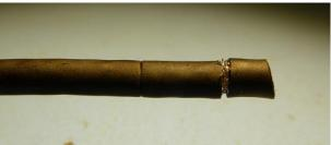
5) Remove the outer cable sheath and braided shield.
