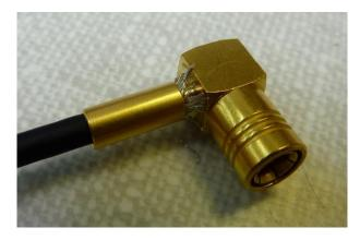
16) Using the pick, tuck any excess shield into the crimp. Push the crimp up to the connector body. The crimp must be flush to the connector body, with no strands of shield showing.
