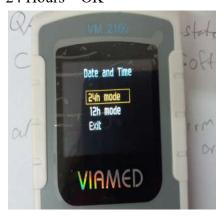
Set/Check Date – press twice for each digit – cycle through each one and correct the date and time if needed. (the time is usually and hour out)
