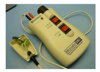
27) Using low-melt glue, affix the PCB into the case.
