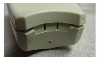
7) Using a reaming tool, enlarge the hole to 6mm to fit the strain relief.
