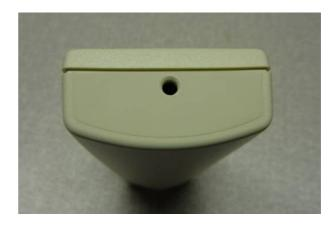
3) Using a reaming tool, enlarge the hole to 10mm to fit the BNC connector.
