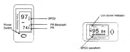
It is apparent the heart rate bargraph display corresponds with pulse rate.
