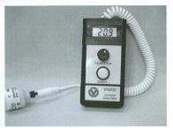
The left hand comer of the display indicates a battery symbol when batteries are low. The front panel contains the ON/OFF push button and the calibration control. The instrument incorporates an auto switch off. Upon receipt inspect the entire unit for damage. If damaged do not use. Notify the supplier or consult Vandagraph. The analyser can be supplied on request with the auto-switch off disabled.
