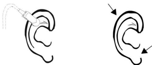
**EN:** Measurement position without cable support
