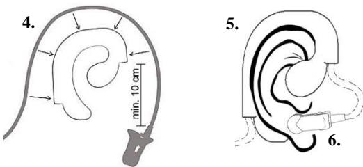
**EN:** Insert Ear sensor into cable support and connect to ear
