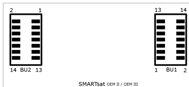
Figure 3-6: BU1 and BU2 PIN OUT (OEM II and OEM III), Bottom View
