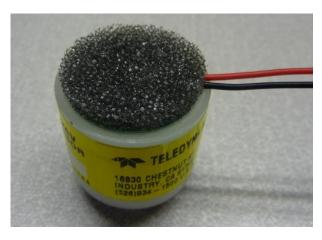
14) Noting the serial number, remove the sensor label.
