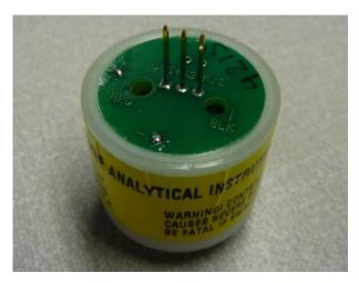
4) Using a soldering iron and pliers, remove the pins.
