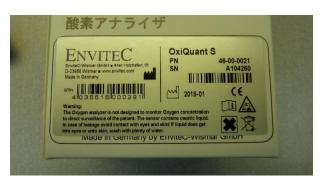
Check the serial number of the Oxygen sensor, which can be found on the white label near the sensor base.
