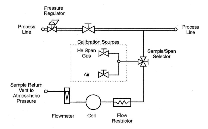
Figure 2-3: Typical Sample System with Provisions for Calibration
