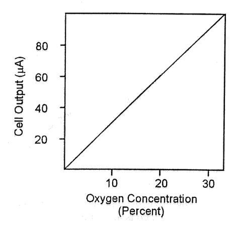
Figure 2-1: Characteristic MFC Input/Output Curve Typical of a Percent Oxygen Cell
