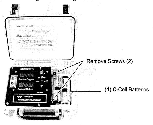
Figure 3-6: Battery Installation
