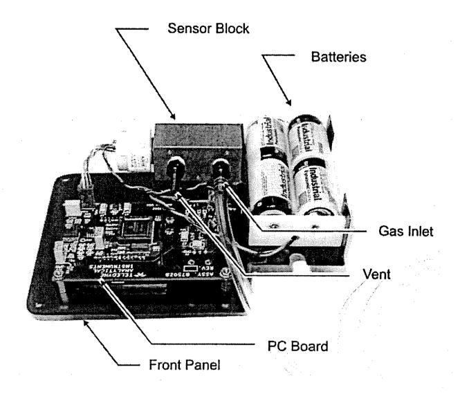
Figure 2-2: Internal Components
