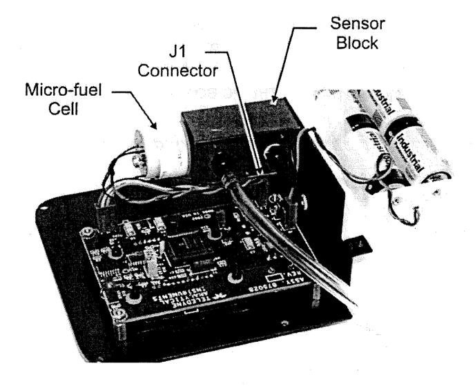
Figure 5-1: Replacing the Micro-Fuel Cell
