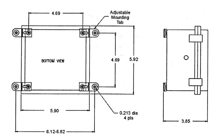
Figure 3-1: Mounting Dimensions
