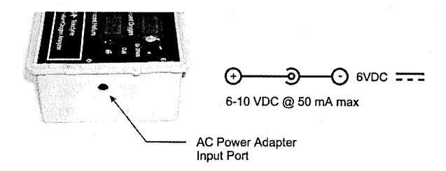
Figure 3-4: Power Adapter Port (Wall Mount)
