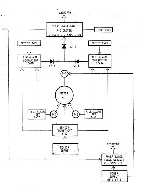
S-1: HIGH ALARM CHECK S-2: LOW ALARM CHECK S-3: BATTERY CHECK
