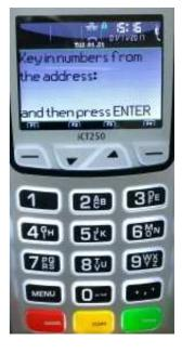
When the details have been entered, the machine will attempt to connect, this may take a minute or so to complete.
