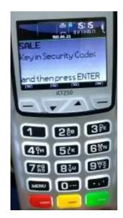
Enter the numerical digits from the postcode as per card slip 2, and then press the green 'ENTER' key.
