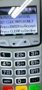
As instructed, tear off the receipt. If it has printed correctly, press the green 'ENTER' key or press the 'MENU' key to reprint.
