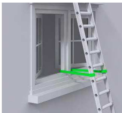
Figure 6 Correct – ladder tied at top stiles (correct for working on, but not for gaining access to a working platform/roof etc)
