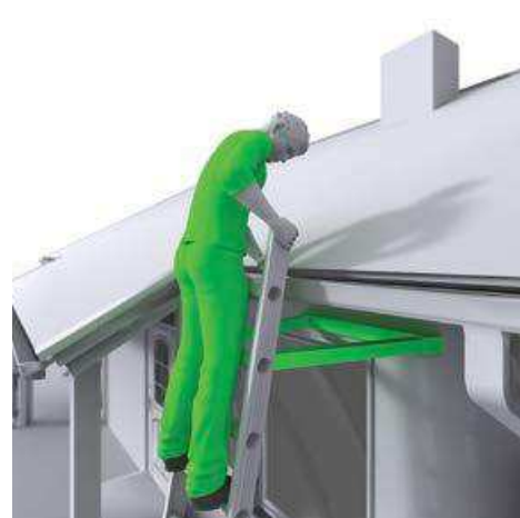
Figure 4 Correct – use of a stand-off device to ensure a strong resting point. Do not rest a ladder against weak upper surfaces such as glazing or plastic gutters. Follow the manufacturer's instructions
