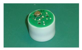
4) Insert a grommet into the hole in top cap.
