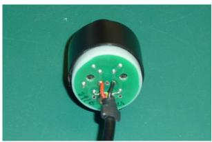
14) Apply a modest amount of super glue to the inside of the sensor cap. Firmly press and hold the sensor cap in place. Wipe away any excess.
