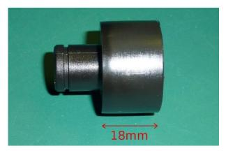
11) Apply clear adhesive silicone to the inside face of the sensor housing.
