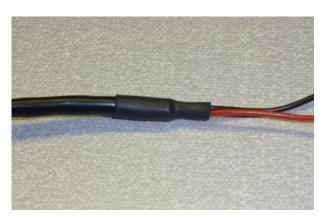
22) Affix a ferrite by looping once thought. Leave 60mm of sheathed cable protruding from the ferrite.
