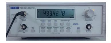
Example shows reading at 120 bpm, i.e. target value 500.00 ms.
