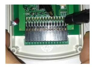
If measured value is not displayed it may be necessary to slightly adjust the DC THRESHOLD/AC COUPLED OFFSET.
