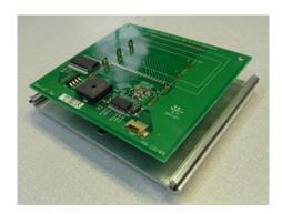
Ensure that the PCB is flush to the battery compartment, then solder the contacts to the PCB.
