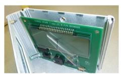
Follow the steps previously mentioned in the keypad replacement section to reassemble.
