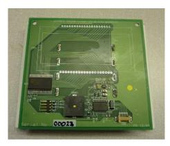
Locate the display orientation markers on the PCB and LCD.
