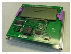
Solder the LCD to the PCB then remove the supports.
